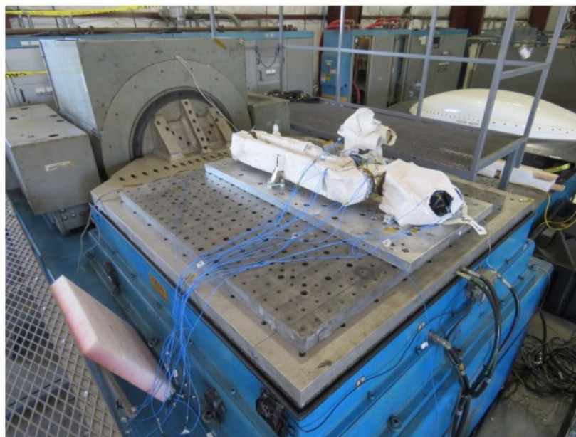
Z-Axis Vibration Test Setup
